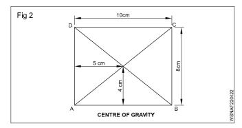
3 A thin lamina is shown in the figure below. Find the centre of gravity.
