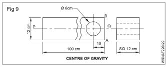
Volume of rod =  $a^2h$  unit<sup>3</sup> =  $12 \times 12 \times 100 \text{ cm}^3$ =  $14400 \text{ cm}^3$  Volume of circle =  $\pi r^2 h$  unit<sup>3</sup>
