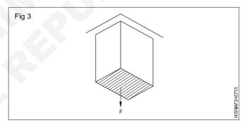
$$\frac{\text{Ultimate stress}}{\text{Working stress}} = \text{Factor of safety} = 4$$
