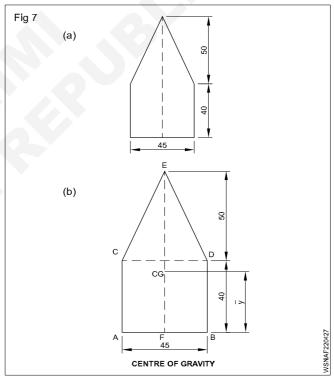
As the body is symmetrical about y-axis centre of gravity lies on this axis.
