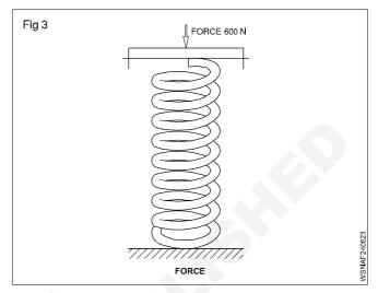
4 Helical spring is loaded with a force of 400 Newton and it is compressed by 18 mm. What would be the load required to compress it to 6 mm?
